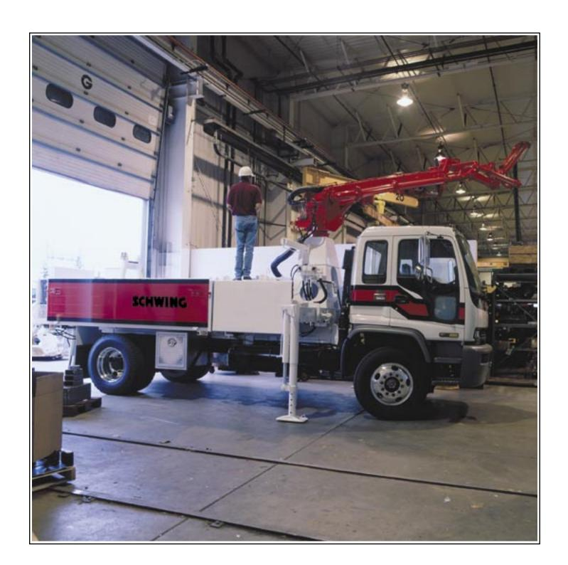
Maneuverability on-site and economical single-axle truck mounting are the obvious benefits of the KVM 17. With a low 16'4" unfolding height for warehouse flat work and all the features of larger Schwing boom pumps, this
