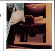
Completely sealed waterbox for flushing cylinders features easy access for inspecting and changing pumping rams.
