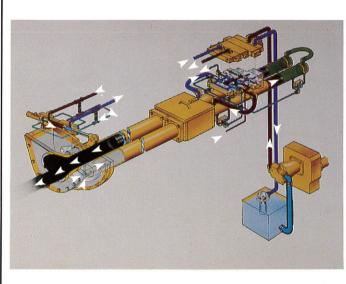
The BPL 1200 HDR is equipped with a hydraulic system which can be changed to provide greater volume of concrete or greater vertical and/or horizontal pumping distances. Hydraulic pressure is applied to the rod side of the cylinder piston head for greater volume or to the face of the piston head (high pressure side) for greater distance. This feature is only available on Rock Valve equipped units used for line pumping.
