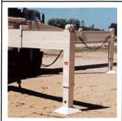
Fully hydraulic outriggers for fast and simple set-up and excellent stability in all boom positions. Outrigger controls are located on opposite sides of the unit. Operators can observe outrigger extension during set-up.
