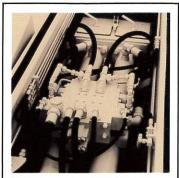
Hydraulic control block is the proven Schwing design providing millions of hours of service. This simple foolproof unit switches hydraulic flow without troublesome electronic devices.
