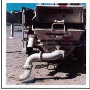
Convert your Schwing from boom pump to line pump with the addition of a simple 90-degree outlet. This allows full utilization of the pump for high-pressure, long distance placements.
