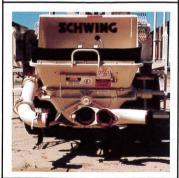
Discharge pipe swings away for fast, effective cleaning of the Rock Valve and housing. Convenient hinged clean-out doors are also incorporated.
