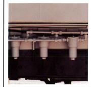
Easy access hydraulic filters screen down to 10 microns to protect system from contaminants.
