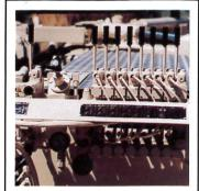
Controls for boom and pump are conveniently located for easy operator access on the pump's wide deck.
